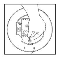
b. Turn the thumbscrew and open the hinged door located inside the back box.
